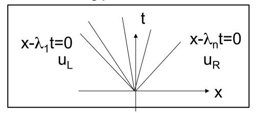
The solution consists of m waves emanating from the origin. They constitute the wave fan. Each wave carries a jump discontinuity.
